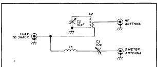
fig. 2. This 2-meter diplexer will permit use of the same coax feeder for a separate 2-meter antenna without compromising performance on either 144 MHz or the lower bands. Both L2 C2 and L3 C3 are carefully tuned to 144 MHz. The link on L2 is one turn. L2 and L3 can be 4 turns No. 18, 1/2-inch diameter, 3/8 inch long.
