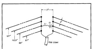
fig. 1. Electrical dimensions of the 5-band dipole. L1 and C1 are used only for 2-meter matching. C1 is 2.2 pF ceramic and L1 is 3 turns of No. 12 wire, 2-inch inner diameter, 1 inch long, air wound.
