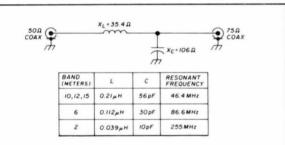
fig. 5. This simple L-section will provide a broad-band match between 50 and 75 ohm coax. Target values for the inductive and capacitive reactances are 35.4 ohms and 106 ohms, respectively, but values are not critical. The bandwidth is so broad that the 15, 12, and 10 meter bands can be covered with one fixed L-section. If the 50-ohm port is shorted the inductance can be adjusted with a grid dip meter to the frequencies shown in the table.
