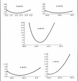
fig. 4. SWR curves measured on 75-ohm coax. The antenna was matched at the low end of 6 and 2 meters where all operating for this particular station is done.
